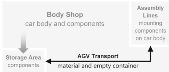
Fig. 3.5 Schematic representation of production and AGV transport of components
